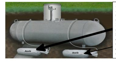
A Sacrificial Magnesium Anode is buried alongside the tank, then connected through a set of wires. Replacing the anode simply requires digging 2 small holes alongside the tank, disconnecting the wires from the failing anodes, then connecting the wires from the new anodes.
